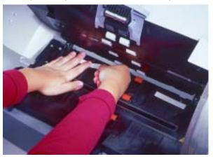
14. Lower the scanner door and press it firmly until it snaps into place.
